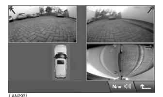
Selecting **Proximity View** will display a combination of three images from the front and passenger side cameras. These views give the driver an enhanced view of the area forward and opposite the driver.
