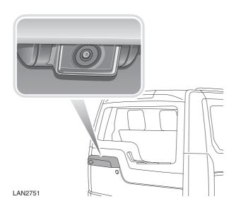
The rear view camera system provides a rear view image to assist in reversing the vehicle. Overlaid on the image are reversing guidelines.
