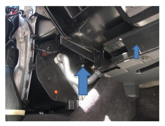
Hopefully the motor you're after is on the passenger side, because the driver's side ones are a *nightmare* to get to. Access probably could be vastly improved by removing the plastic surrounding the steering wheel (small arrow, above). However, I believe that total removal involves taking the steering wheel and steering column controls etc off, so now its decision time.
