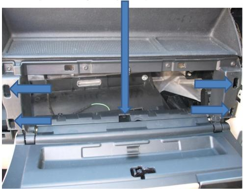
8. ... and here's the clip that makes withdrawing it difficult
