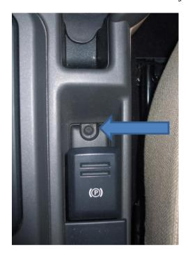
15. Remove the rubber sunglasses holder, then the plastic bit underneath it. A hidden Torx screw should be found underneath. Very cunning Mr Land Rover.
