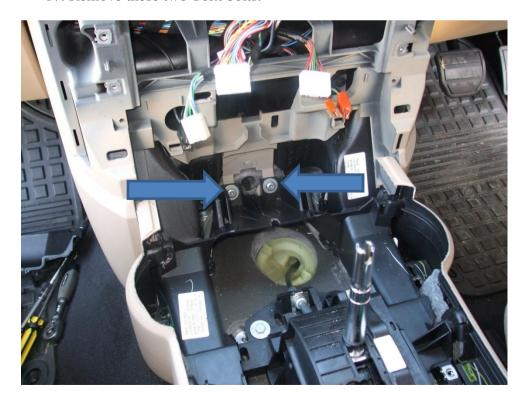
18. Raising the console at the rear slightly, slide it backwards as far as it will go. Because I never found a way of disconnecting the wiring loom indicated it will only go so far.
