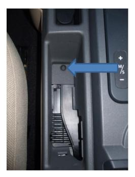
Now pullwards up the top section of the console. A lot of plastic breaking sounds will be made that sound expensive. At least one clip of mine is permanently broken. I don't think there's any trick here, just luck.
