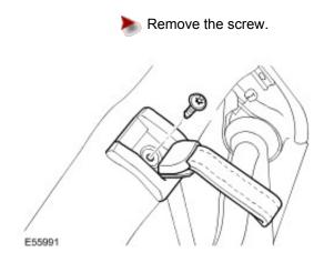
5 . Remove the seat front release strap finisher. Remove the screw.
