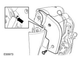
4 . Remove the seat rear release strap finisher.
