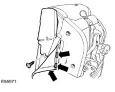
3 . Remove the rear seat cushion side finisher.Remove the 2 screws.
