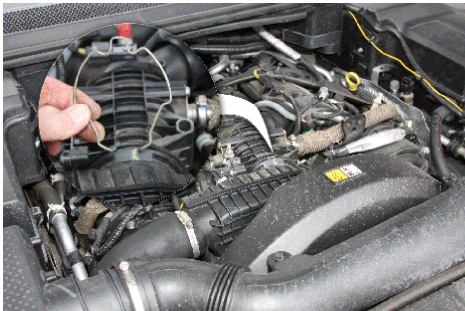
Air box to EGR butterfly housing securing clip
