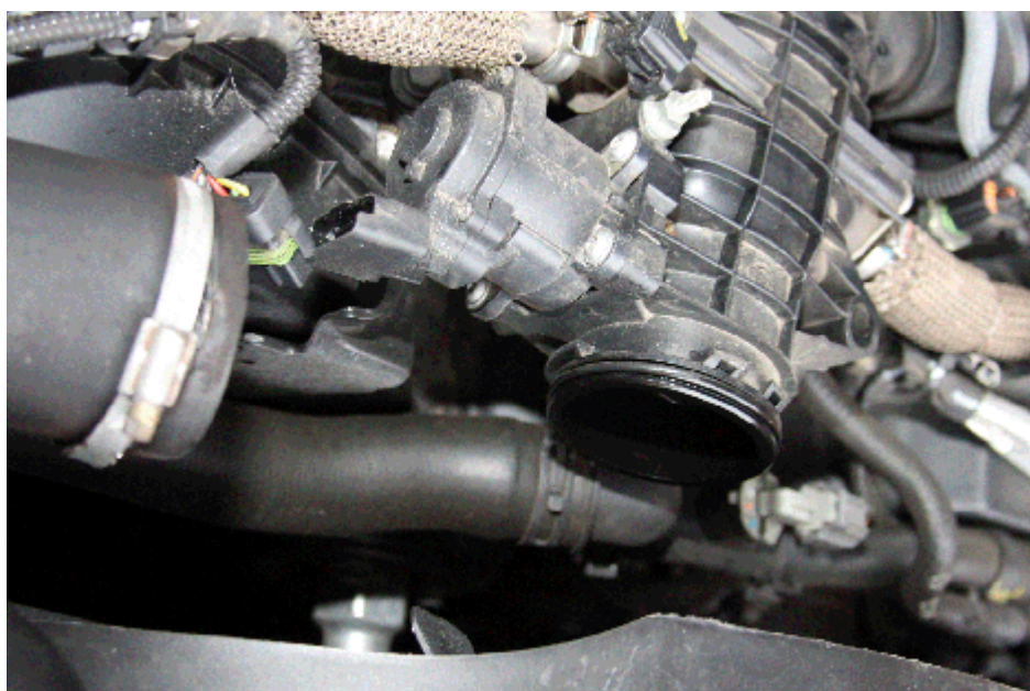
Air box removed
