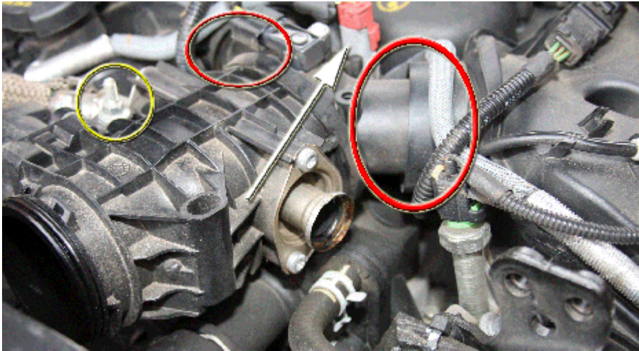
Raising the butterfly housing. It will swivel where circled but don't go mad or you'll break whatever is holding the connector(arrowed) to the back of the 'Y' shaped duct like wot I did!
