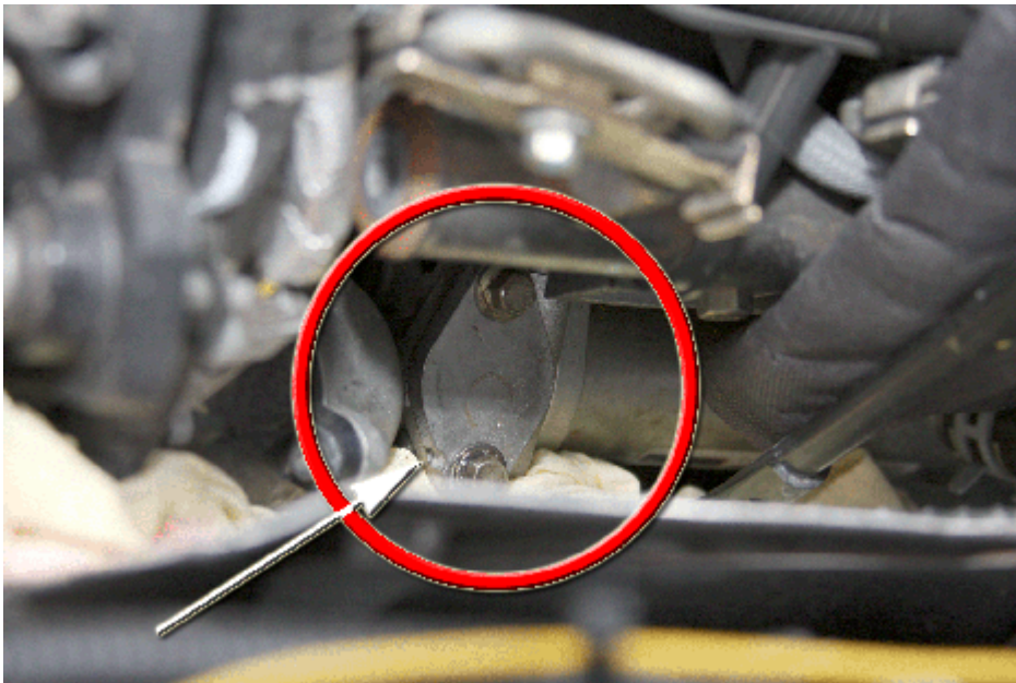
EGR valve blank fitted – indent arrowed!
