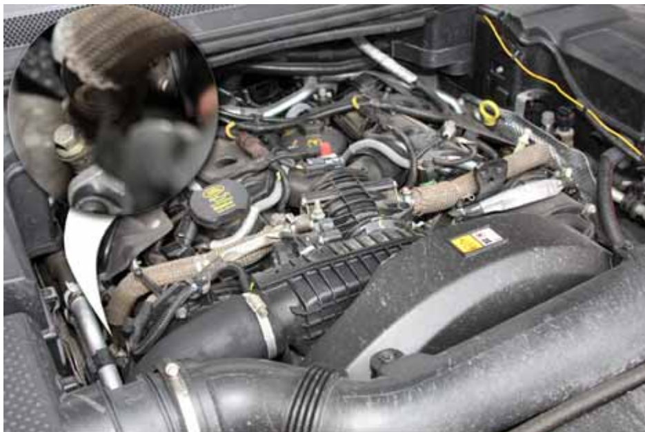
View of engine with top cover removed – right hand EGR valve shown in inset
