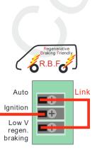
How to connect? Connect ignition feed to the ignition terminal. Link Auto to Low V with bridge cable. Double all voltages for 24V, triple for 36V and quadruple for 48V.
