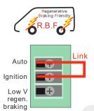
How to connect? Link the Auto and the Ignition terminals on the block together, as shown.
