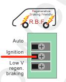
How to connect? Connect ignition feed to the Ignition terminal. Can be any live feed.
