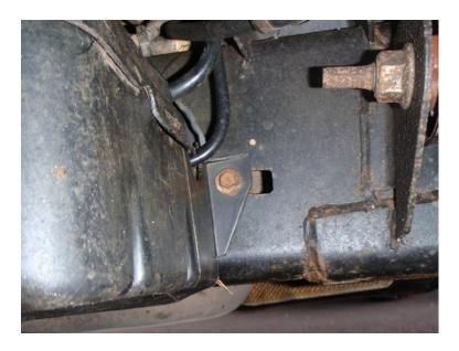
Also remove the bolt that secures the lower cover to the compressor using 10mm socket/spanner . This goes straight up from underneath the cover (RH hole in picture. Mine has sheared off so isn't there anymore). LH hole is the drain hole
