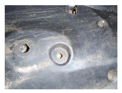
Release the four clips that secure the lower cover to the upper cover. There is one towards the front of the vehicle, one towards the rear and two on the side.
