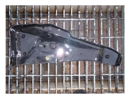
I also enlarged the existing drain hole to 25mm and drilled a new 25mm drain hole
