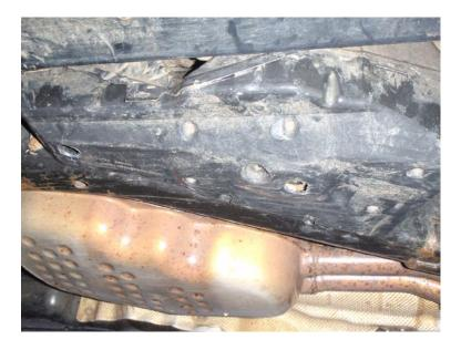
With the foam removed and the extra drain holes the mud etc should drain a lot clearer and quicker. In addition, a hose pipe can now be presented through the drain holes to assist future cleaning without the need to remove the cover.
