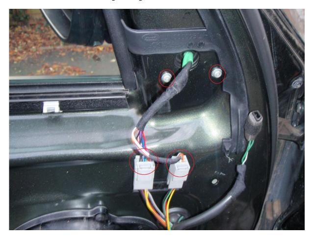
7) With the screws removed the wing mirror can be removed from the door.
