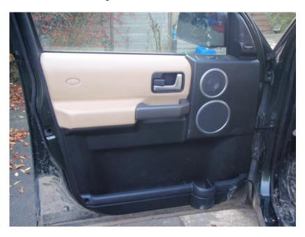
1) Unclip the 4 clips on the door handle. There are 2 clip on the top and two clips on the bottom. A small screw driver can be used to loosen the handle. Once the two bottom clips are loose, lift the handle upwards. Some force is required but too much and the clips can break resulting in a new door handle.
