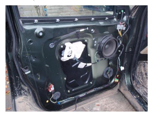
6) With the panel off you then need to disconnect the two wing mirror electrical connectors and undo the 3 Torx screws securing the wing mirror.
