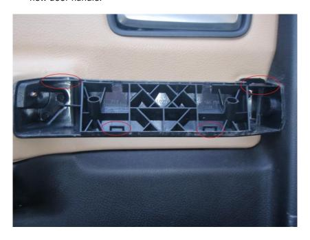
2) Remove the two screw covers and undo the 8 screws (Phillips) holding the door panel
