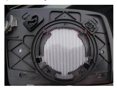
You then need to push the glass in and down to secure. This was the tense moment as too much pressure and the glass could break.
