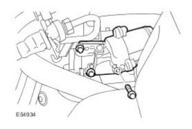
14 . Remove the RH exhaust manifold heat shield.
