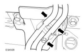
7. Disconnect the EGR valve electrical connector.
