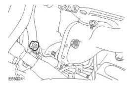
16 . Remove the remaining exhaust cross-over pipe nut.
