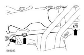
15 . Remove the 2 exhaust cross-over pipe nuts.
