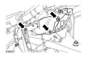
13 . Remove the RH EGR valve and cooler assembly.
