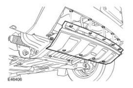
The front towing/lashing eye is accessible after releasing the 9 toggle fasteners securing the towing eye access panel and removing the panel.
