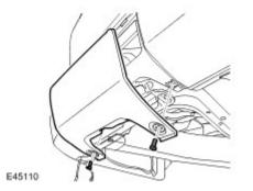
The rear towing/lashing eye 'A' is accessible after releasing the 2 fasteners securing the access panel to the bumper and removing the panel.
