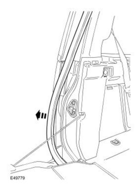
5 . Remove the support spigot from the tailgate. Release the clip.
