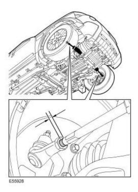
13. If the steering wheel is more than three degrees from the straight ahead position, remove the steering wheel and reposition on the nearest spline to the straight ahead position.
