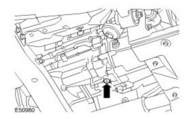
7. Install a new transmission fluid drain plug and tighten it to 35 Nm (26 lb.ft).
