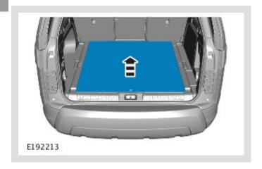
Remove the load space floor panel.
