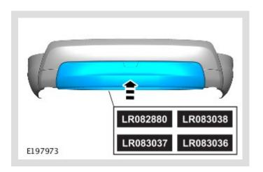
Install the deployable towbar cover.
