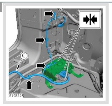
Connect the electrical harness to the towbar module.
