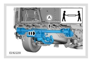
With the aid of another person, install the deployable towbar.
