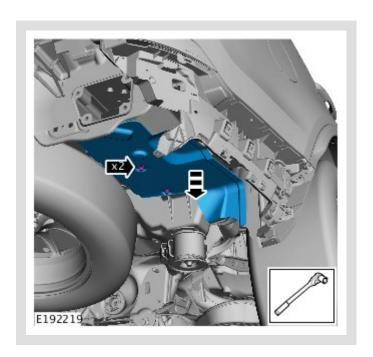
Remove the muffler heat shield.
