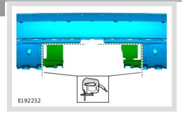
Using a suitable tool, cut the rear bumper as illustrated.
