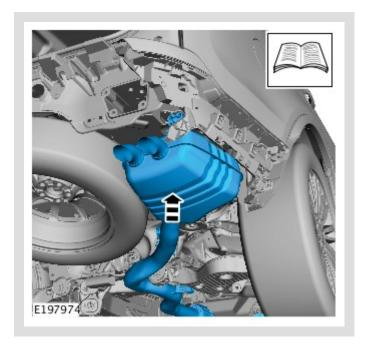
Install the rear muffler.
