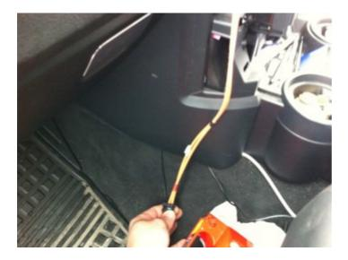
Next , undo the 2 screws holding the passenger side trim in place ( screws are just below the bottom glove box)
