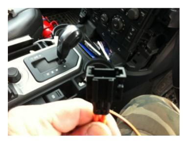
Plug that into the end you removed from the nav screen ( blue tape )
