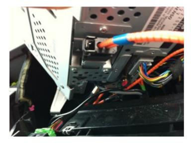
Put the nav screen back in place and make sure the end of the most cable ( red tape ) is coming out of the top left of the screen
