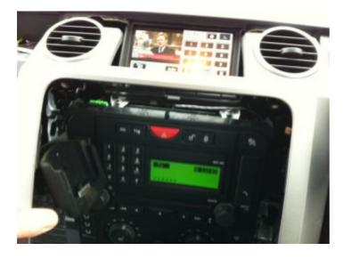
Next remove the 4 screws holding the nav screen in place
