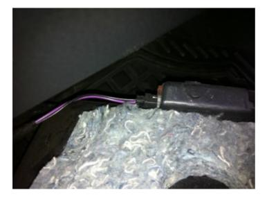
The bit that fits in the far left hand side is just a plastic tab , you will need to wiggle it to get it out ..or undo the trim thats holding it in place ( undo the screw holding the bonnet release , and pull the trim towards the front seats )
