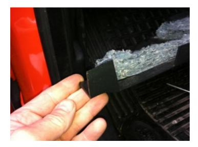
When its out the way , there is a screw holding the bottom part of the center consul in place .Remove this
