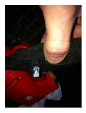
Pull the trim out wards , and undo the connector for the light ( just pulls outwards)
