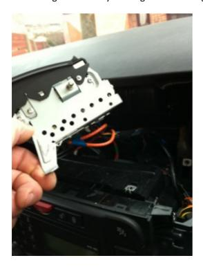
Undo the connector by pressing the clip in at the side and pull out the connector
