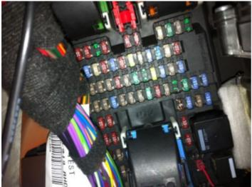
This plugs into the fuse box in fuse 58. The original fuse goes back into the new piggy back fuse holder and i would use a 3 or 5 amp for the Bluetooth module .
