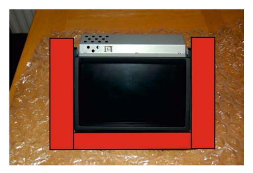
The "H" trim now need to cut right along the bottom edge where it butts up to the bottom of the screen, you might also need to remove a small amount of material from each side of the "h" trim that's butts up to the screen sides.
