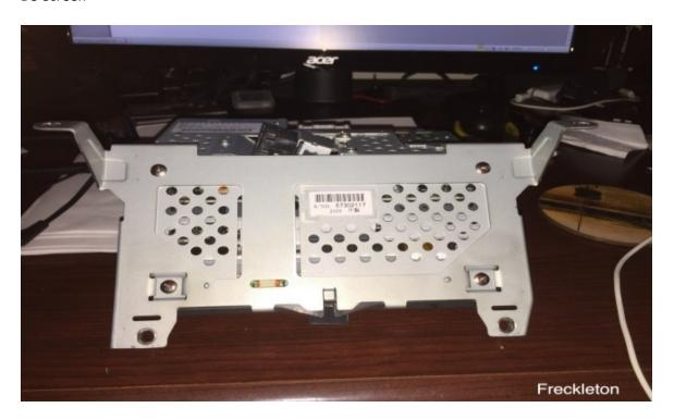
Now lay the D3 screen mount over the D4 screen mount and mark the four screw holes in the D4 back plate to be drilled, make sure you have the back plate the right way up. You don't have to be exact but ensuring the front holes where the screen mounts in the D3 are in the same position, these are the holes that hold it in the car.
