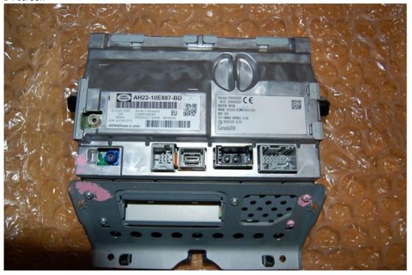
Now do the same on the D4 screen, by removing the back plate as shown below by removing the four screws.
