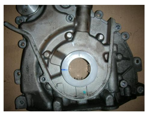
In this picture you can see the oil pump drive, I have moved it to one side so it can be seen.
