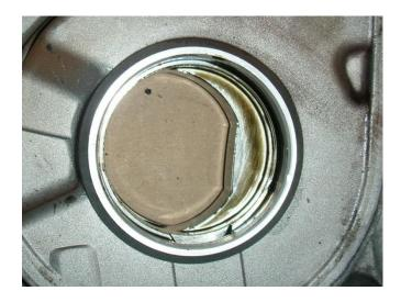
Clean all surfaces and lightly grease the rubber gasket on the casing and on the sump. I also filled up the oil pump drive chamber with clean oil to help prime the system before I started the engine.
