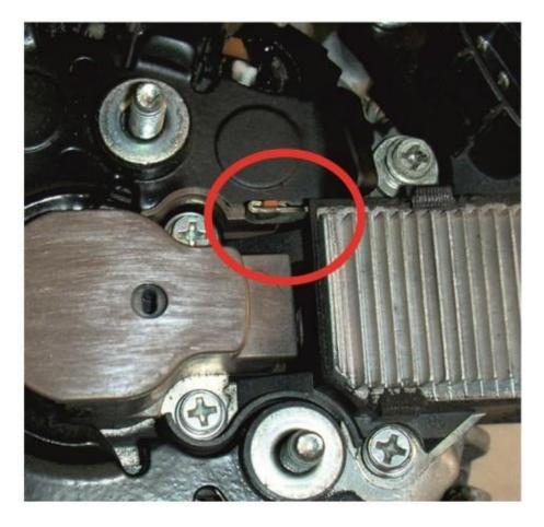
As you can see in the picture below there are two diodes that have blown apart there was a total of 5 that where in this condition.
