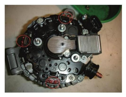
Once you have removed the solder you can now remove the diode pack from the main body of the alternator by lifting it off the three studs, you should now have this view.
