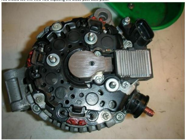
Now remove the two screws holding the brown carbon brush holder in the centre of the unit, then just lift it off and put it somewhere safe out of the way.
