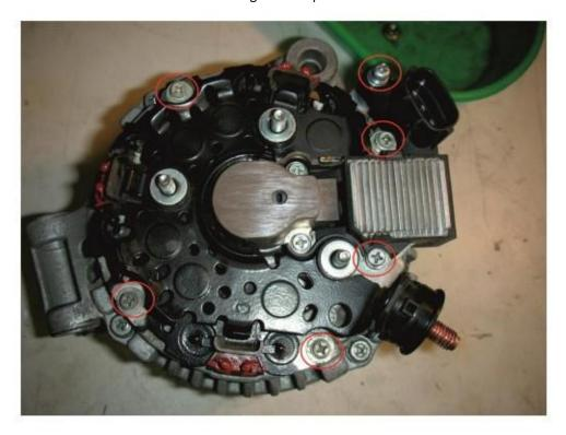
Once removed store in safe place. Also remove the black plastic bobbin on the main battery lead terminal and store in a safe place.
