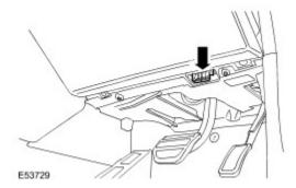
3. Start the engine. Move the selector lever from 'P' through all gear positions, pausing in each gear position for 2-3 seconds and return to the 'P' position.
