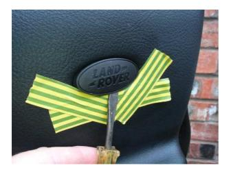
You don't really need the protective tape as it's quite loose anyway & covers the screw for the door. It has a plastic tag to hold it in place.
