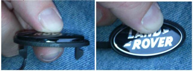
The solution is to shave off some of the plastic in two dimensions. 1<sup>st</sup> is the height (thickness) that needs to reduce
