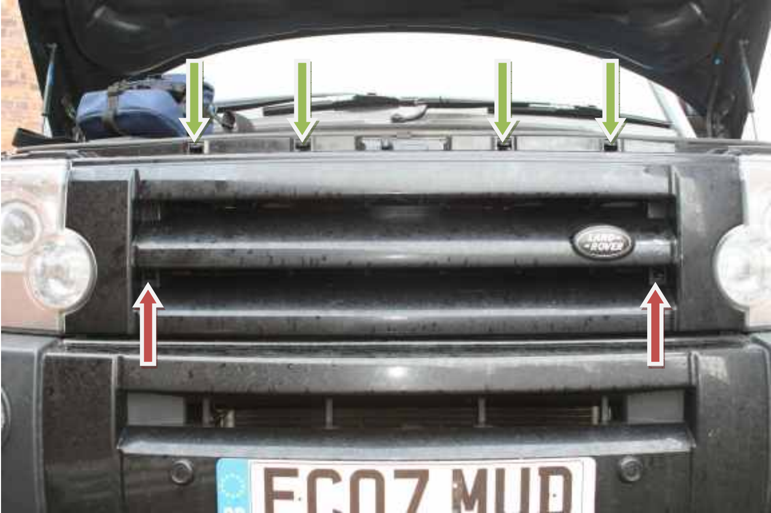
Push down where the green arrows are, Lift up where the red arrows are.
