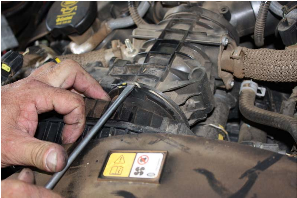
Remove clip holding intake box on inlet manifold (insert screwdriver and twist)
