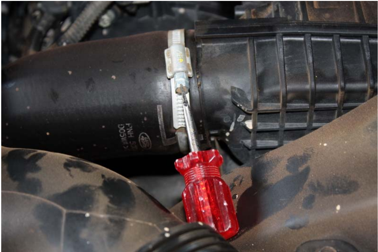
Loosen jubilee clip on intercooler pipe
