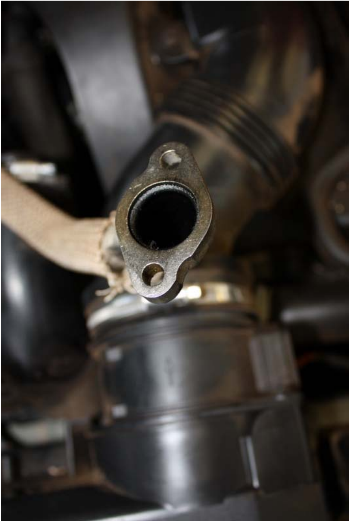
Clean up EGR pipe face
