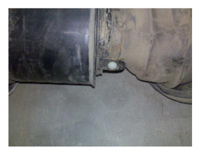
The next step is to release the collar of the airspring from the body of the shock itself.Unfortuneately I don't have a picture but its very simple to do.With the lower part of the shock held in a vice, using a piece of timber and a hammer gently tap the rounded end of tab arrowed below
