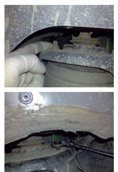
As you lower the spring the airline will pass down through a hole in the top of the turret. You can now remove it completely. Make sure and cover the hole & the end of the green pipe with some tape
