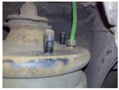
**Airspring Removed :** With spring removed , in order to move further you have to remove the protective rubber gaiter from the airspring. I just cut it immediately under the retaining band with the metal casing underneath lessening the risk of slicing through the airbag below. Then pull the gaiter down to reveal the inner workings.
