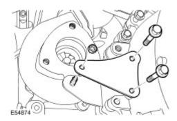
10 . Remove the turbocharger support bracket retaining stud.
