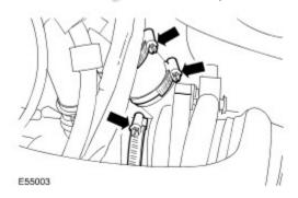
26 . Disconnect the turbocharger electrical connector.
