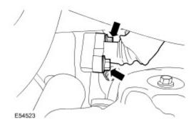
23 . Remove the turbocharger securing bracket.
