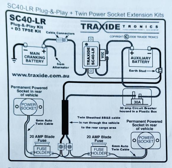
This kit is designed to add two new permanently powered cigarette lighter type power sockets to the rear of a D3 and the kit is designed to be connected to the Auxiliary Battery fitted in the engine bay.
