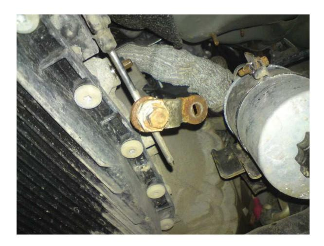
If you are just going to clean up the bush, you may even manage to leave the bolt part on the cable and remove the rest of it to a vice.
