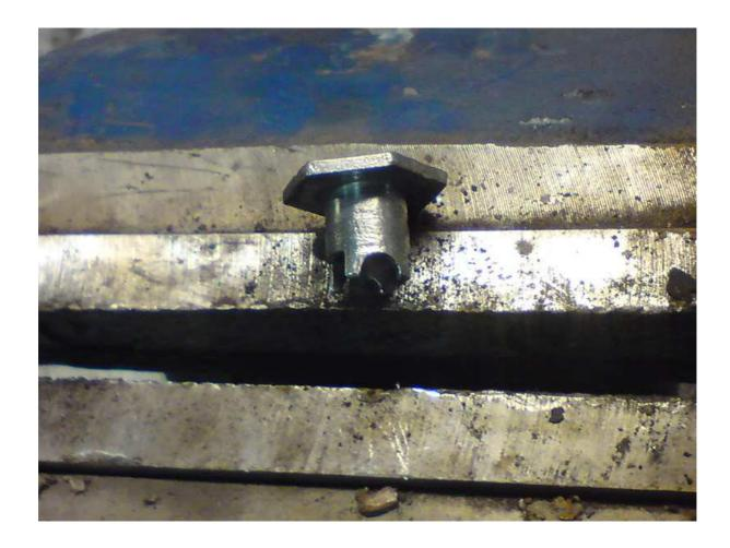
The bush has a square section and a smaller rounded section. The square part of it holds the head of the bolt in place, and the smaller part clamps the cable in place. It is vital again that these are correct otherwise you risk bending the cable and breaking the insert. Grease the bush and place into new arm, refit to selector cable and fit both 13mm nuts loosely, ensuring bolt is lined up correctly.
