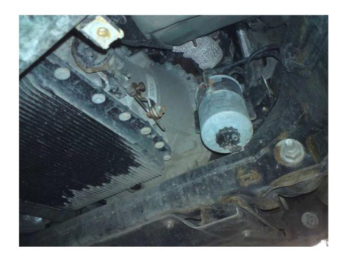
Locate selector lever and remove the top nut. It is important that the top one is undone first, otherwise you risk twisting the shuttle valve out of the valve block, and requiring the sump to be removed and your gearbox internals stripped
