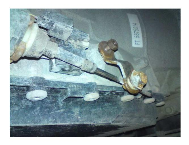
Before removing the top nut completely, hold the metal part with a 21mm spanner, and undo the lower 13mm nut securing the cable to pivot arm. Once it's loose, remove the top part from the gearbox and then remove the lever from the selector cable.
