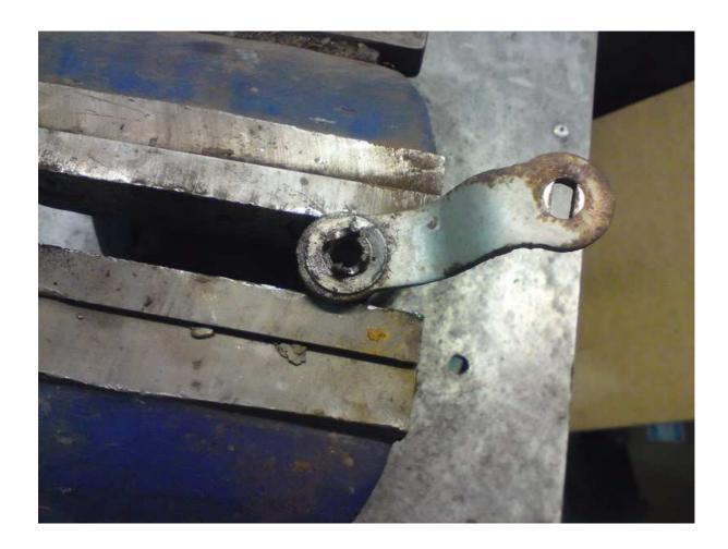
Hold the hex part of the metal insert and twist it and apply pressure upwards to remove the plastic bush from the metal insert. Once removed, bin the arm, and you are left with the bush.
