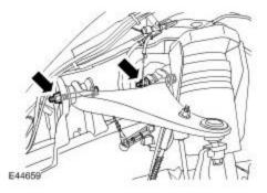
6. Disconnect the height sensor link arm.
