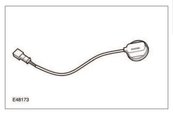
A single microphone is used for hands-free telephone operation and for the voice recognition system. The microphone has an integrated noise suppression system for hands-free telephone use. The microphone is a standard directional type and is located in the front roof console.
