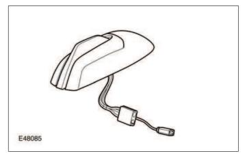
The Cellular Phone Antenna is located in the roof mounted pod and is connected via a single coaxial cable to the TM.
