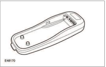
The telephone system allows for the use of different types/manufacturers handsets. This is achieved using a handset specific cradle which is mated to a standard base plate. The design of the adaptor cradle will vary to accommodate different types of phones.
