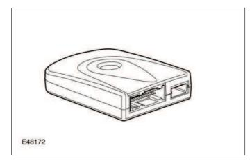
The Transceiver Module (TM) is located in the rear RH quarter of the luggage compartment. The TM is the interface between the telephone and the Integrated Head Unit (IHU). The TM also contains the telephone voice recognition hardware and software.
