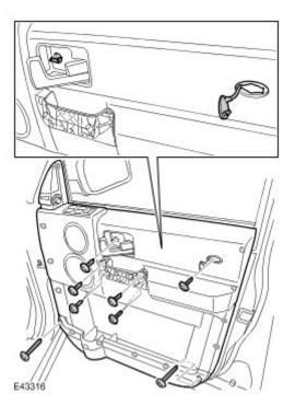
3 . Disconnect the door latch remote release cable.
