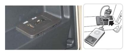
In order to get the full benefit of the **Portable Audio Interface** feature, the harman/kardon hi-line and Premium systems are linked to the touchscreen to provide full control and feedback display. These systems can therefore **only be fitted along with the navigation system**.
