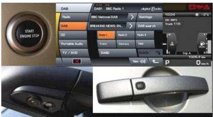
Montage of technology features: Clockwise from top, Push Button Start. Infotainment screen (DAB Radio), instrument pack TFT, Keyless Entry lock buttons, door mirror mounted camera and approach lamps.
