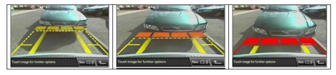
An additional feature for the Discovery due to the mounting location of the rear view camera is **Tow Hitch Assist** which helps the driver to precisely couple the tow bar with a tow hitch. A coloured dot graphic is displayed on the screen representing the tow ball together with a guide line showing the predicted reversing path of the vehicle towards the trailer tow hitch.
