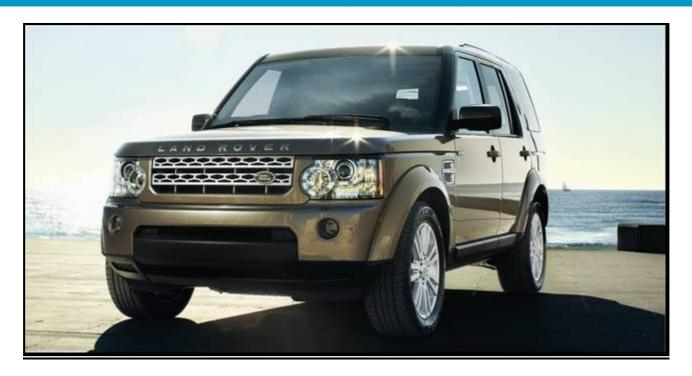
New front wings to accommodate the re-designed front bumper incorporate a side intake on each side necessary for breathing and the twin intake of the new powertrain.
