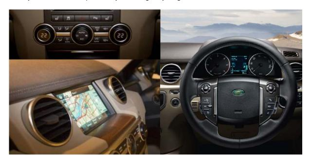
**Memory control switches** for seat and steering column are re-located to driver's door casing for improved accessibility. All models benefit from a new Instrument Panel with a **5" TFT (thin film transistor)** information centre which can display trip information, fuel gauge, primary vehicle information, warnings and supplementary information including In Car Entertainment system.
