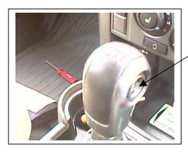
Remove Phillips screws from both sides of the gear knob.
