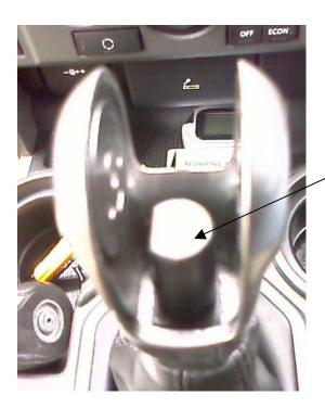
The centrepiece of the gear knob slides out upwards and left with this part.
