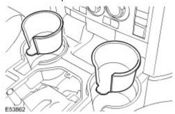
3. Remove the floor console liner.
