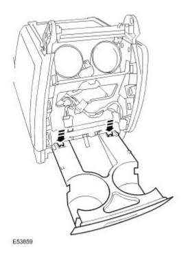
10 . Remove the wiring harness.
