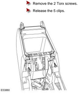
7 . Remove the auxiliary socket panel.
