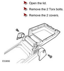
6 . Remove the floor console stowage compartment.
