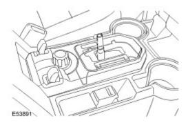
4. Remove the ride and handling optimization switch assembly.
