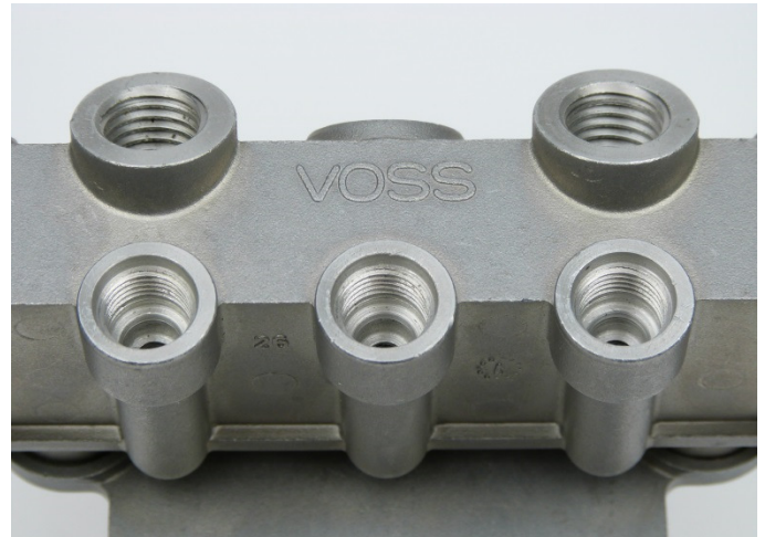
Fig. 11: Clean and correct connecting bores
