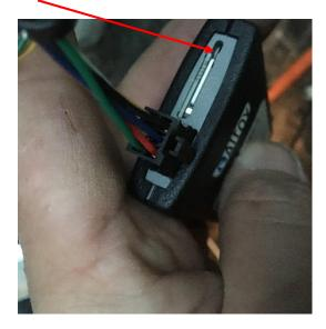
Back to the battery box, connect the trigger wire to the red wire (pin2) on the heater plug, connect the red +ve to the battery terminal, and the ground to the chassis, with all of these in place and tools out of the way, reconnect the battery negative terminal.
