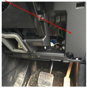
Once hinged to 90 degrees the panel can be pulled away and put somewhere safe, next get a Philips #2 screw driver and undo the two screws that hold the trim panel above the foot pedals
