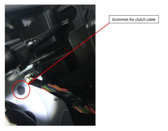
Remove the grommet and push a tool through, I have a range of tools that I use for routing cables, but a Philips screw driver is ideal, you will need to pierce the sound insulation on the inside of the cabin, so it needs a firm push, with this through return to the cabin and look up behind the dash to locate the tool
