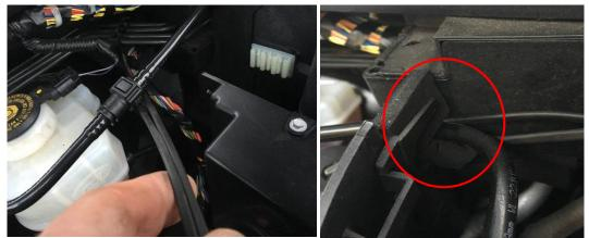
Above the engine at the rear is a cable tray, simply attach the cable to this with cable ties to keep it out of harm's way.
