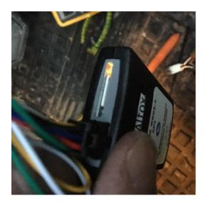
Once happy peal the adhesive backing off the Velcro and stick the unit on the back of the knee panel, to keep dust etc. out I have mounted the unit with the sim slot and wire facing down
