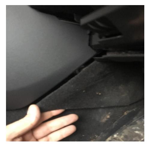
Then finally before removing the panel, disconnect the foot well light, again put this panel somewhere safe out of the way.
