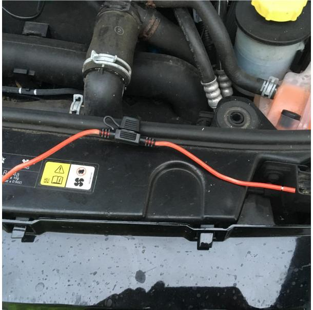
A connection to the cars chassis for the ground or earth, and to run a wire to pin 2 of the fuel burning heater (the red wire toward the front of the plug as pictured)
