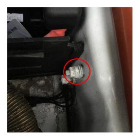
For the trigger wire I have used an inline crimp fitting as I do not want to cut the vehicle wiring loom, (future owners may wish to use the OEM remote system). These types of inline crimps are great for adding a wire and are pretty well sealed once complete, to the trigger wire add the appropriate male connector.
