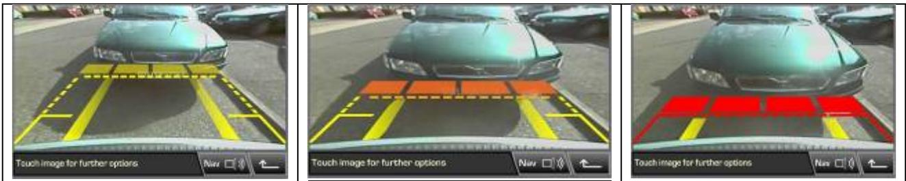
An additional feature for the Discovery due to the mounting location of the rear view camera is **Tow Hitch Assist** which helps the driver to precisely couple the tow bar with a tow hitch. A coloured dot graphic is displayed on the screen representing the tow ball together with a guide line showing the predicted reversing path of the vehicle towards the trailer tow hitch.
