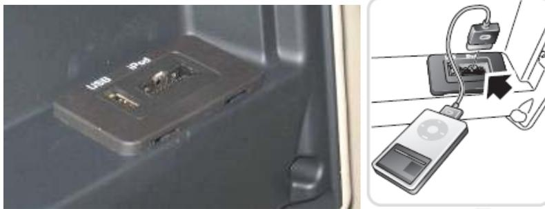
In order to get the full benefit of the **Portable Audio Interface** feature, the harman/kardon hi-line and Premium systems are linked to the touchscreen to provide full control and feedback display. These systems can therefore **only be fitted along with the navigation system.**
