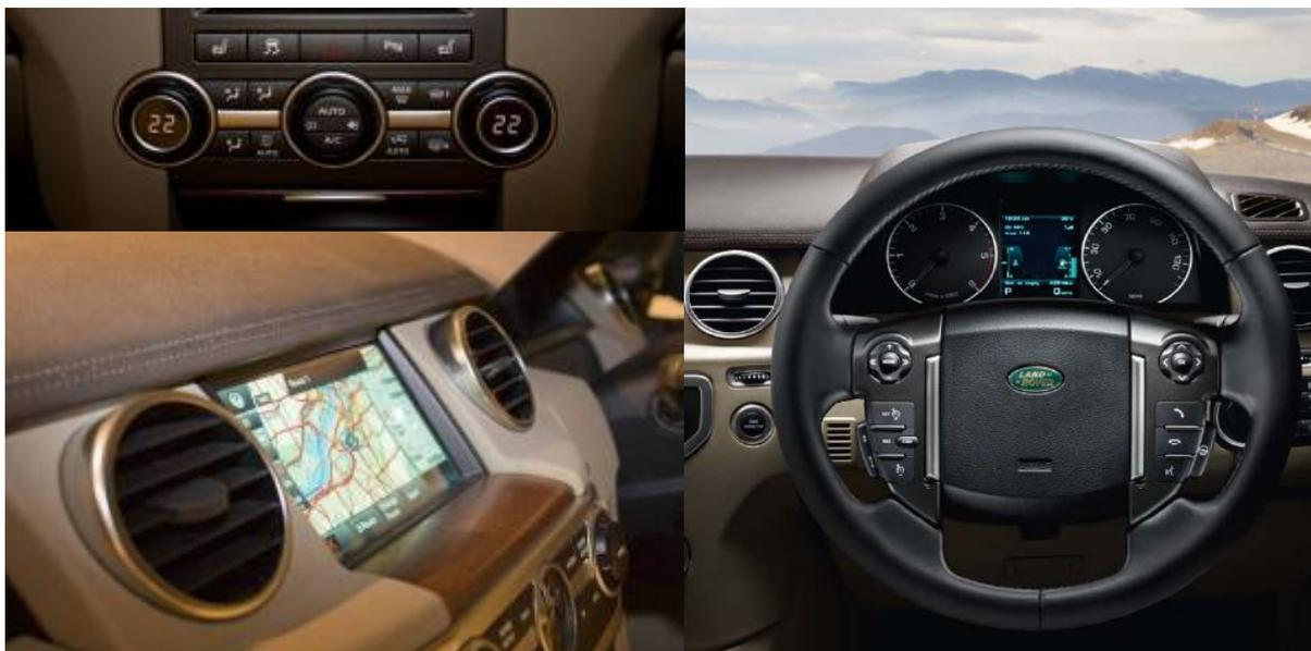
**Memory control switches** for seat and steering column are re-located to driver's door casing for improved accessibility. All models benefit from a new Instrument Panel with a **5" TFT (thin film transistor)** information centre which can display trip information, fuel gauge, primary vehicle information, warnings and supplementary information including In Car Entertainment system.
