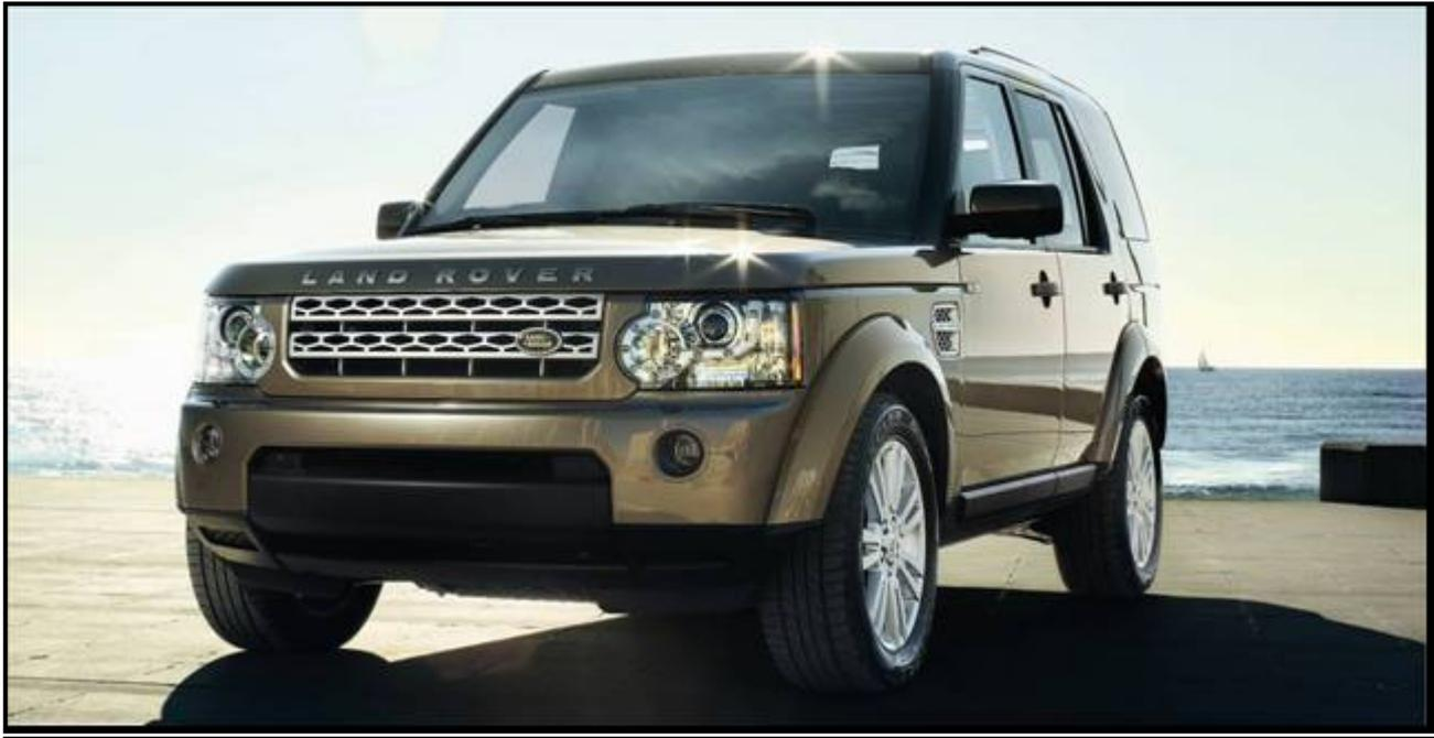
New front wings to accommodate the re-designed front bumper incorporate a side intake on each side necessary for breathing and the twin intake of the new powertrain.
