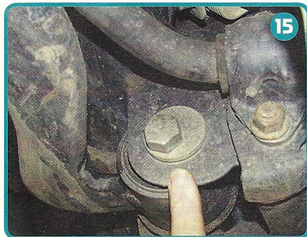
This rear bolt at the extended rear fork of the wishbone moves the fork up or down relative to the chassis to alter the wheel's caster angle
