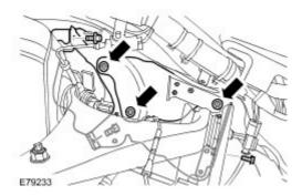
6. Remove the fender splash shield lower trim.
