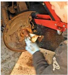
Cleaning up the mating faces where the hub flange meets the driveshaft flange means the two components will go back together squarely. A wire brush followed by 240-grit wet-and-dry paper are ideal for this.
