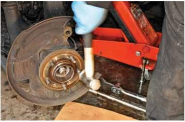
It's quite common for the splines of the driveshaft and the hub to resist separation so, before the hub is unbolted, Rob gives the end of the driveshaft a couple of taps with a soft-faced hammer to release the grip between the two components. This can be done later on when the hub has been unbolted, but this method ensures that the driveshaft actually moves as opposed to the two parts moving together, lessening the effect of the blow. It also stops the hub falling off on to your foot.
