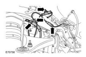
43 . LH side front: Release the 2 air lines. Release from the 5 clips.
