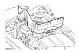
14 . Release the heater pipes.
