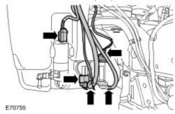
41 . LH side front: Release the ABS sensor lead.
