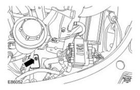
38 . Disconnect the fuel fired booster heater fuel line.
