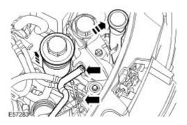
35 . Remove the coolant expansion tank.
