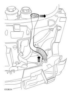
34 . Disconnect the 2 hoses from the coolant expansion tank. Release the 2 clips.
