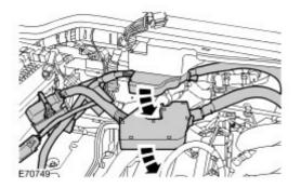
21 . Disconnect the glow plug electrical connectors.
