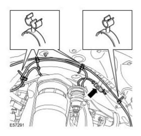
44 . LH side front: Release the integrated body frame ground cables.
