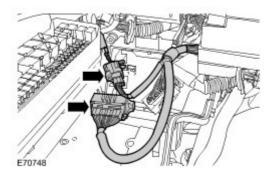
20 . Release the engine and transmission wiring harness cassettes, position the wiring harnesses aside. Release the 2 clips.
