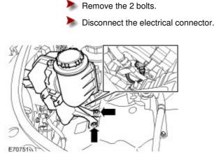
36 . Disconnect the cooling fan electrical connector.
