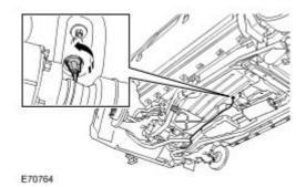
62 . Remove the transmission undershield. Remove the 6 bolts.
