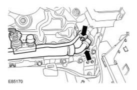
23 . Disconnect the A/C low-pressure switch electrical connector.
