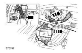
19 . Release and disconnect the 2 transmission wiring harness electrical connectors.
