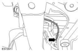
LH side rear: Disconnect the suspension air compressor intake line.
