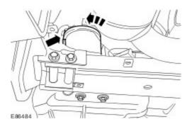
6 . Remove the water-in-fuel sensor.
