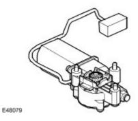
The sunroof motor has a worm drive, which drives a gear in a cast housing attached to the end of the motor. The
