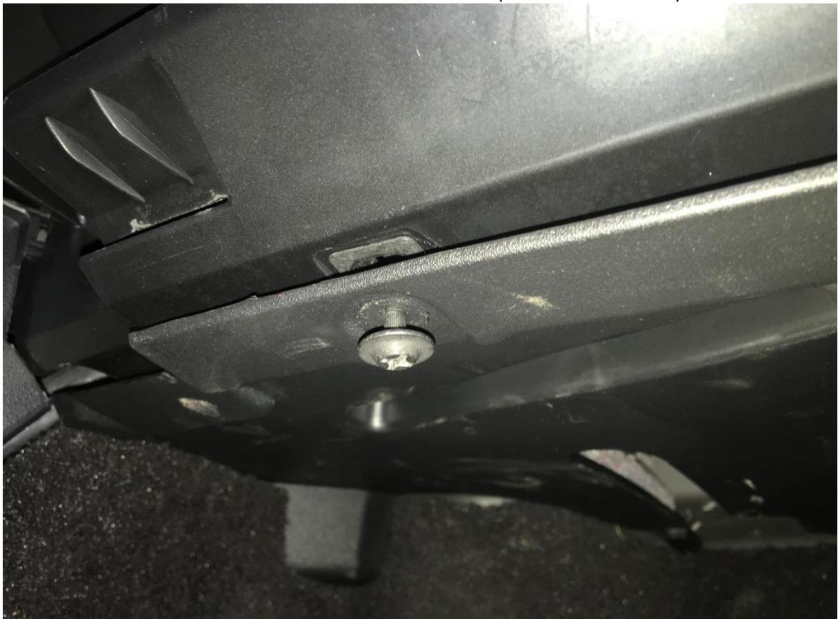
With the screws removed there is a push in clip holding the carpeted end by the central tunnel, pull this way
