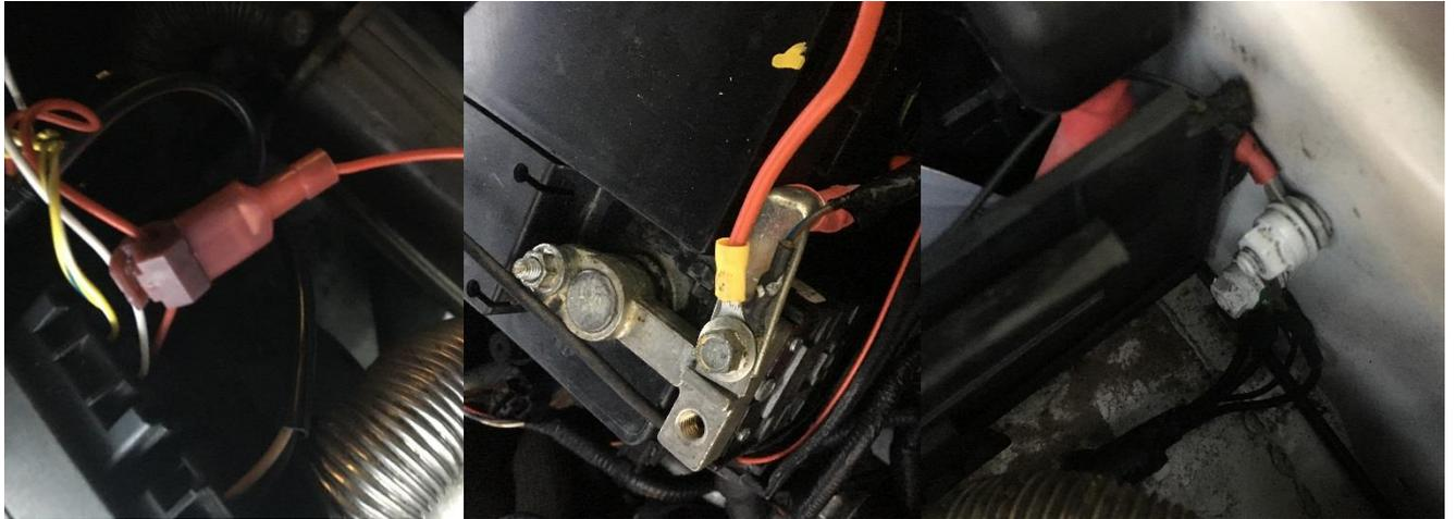
These are the wires that you need to connect to get the unit working and utilise the main functions
