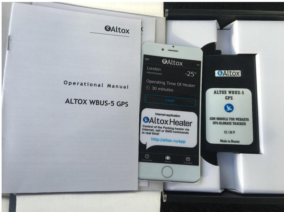
There are two versions of the Altox controller the entry level without GPS, this has the options to control the heater by SMS text messages, simply "START" and "STOP", by voice call to the number of the sim card you have installed, by APP, both Apple iOS and Android and an Altox web based App, so it's far from basic !!!!!
