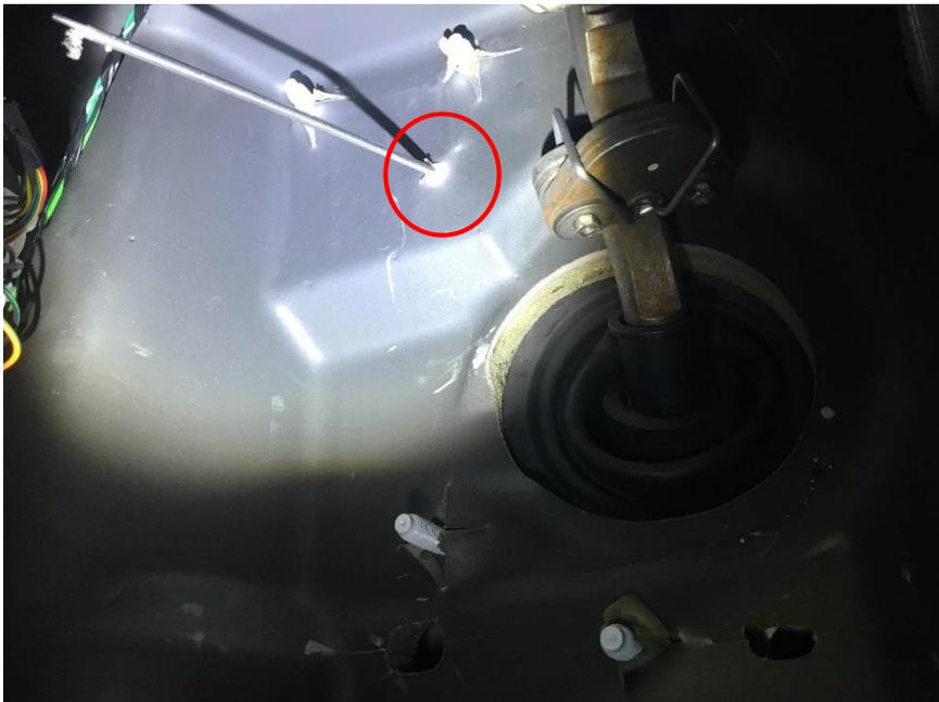
You need to pass 3 wires, so a length of small gauge 3 core cable is ideal, as I have a large roll of 2 core that I use for other installs, I'll be using 2 lengths of that, one for the power feed, and a single wire from the second length for the trigger wire. Attach the wire using electrical tape and carefully withdraw them back in to the engine bay, once through disconnect from the tool and route them
