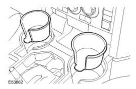
3. Remove the floor console liner.
