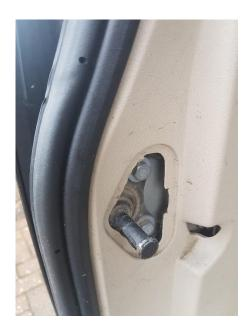
Then, lever the plastic side trim out. It's held in by clips. You just need to ease the rear out, no need to remove it totally. This will give you enough space to access the cable reel.
