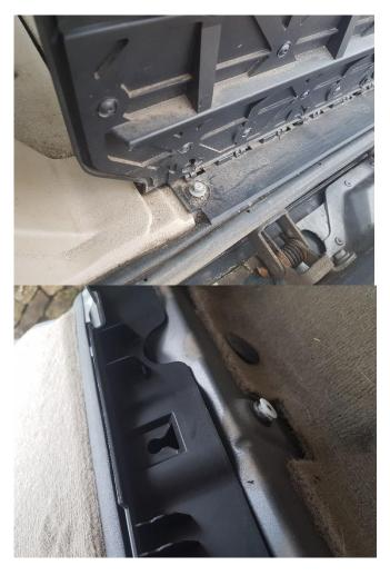
Next, remove the two spring loaded luggage loops on the floor of the boot, one Hex socket (Allen key) bolt each, as these hold down the carpeted trim next to the side trim which holds it in place.
