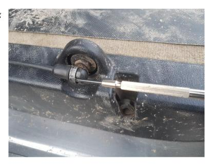
Next, remove the hinged panel flap that extends across the boot over the hinges of the tailgate.
