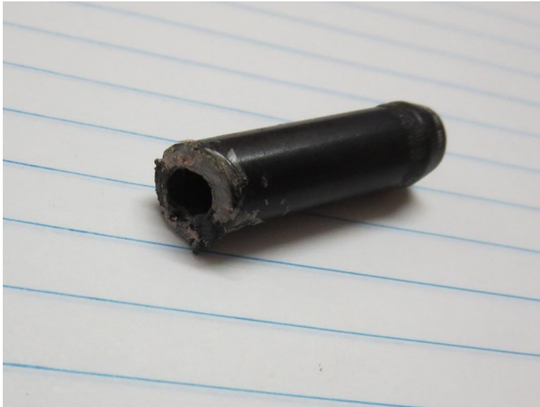
1. Broken fitting. 5mm to 6.5mm tapered I.D.
