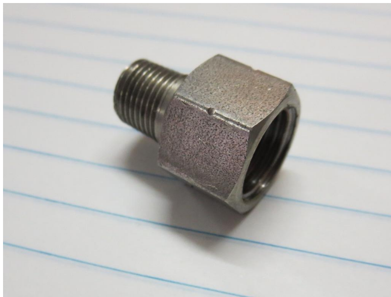
5. 1/4" BSP female to 1/8" BSP male stainless steel reducer
