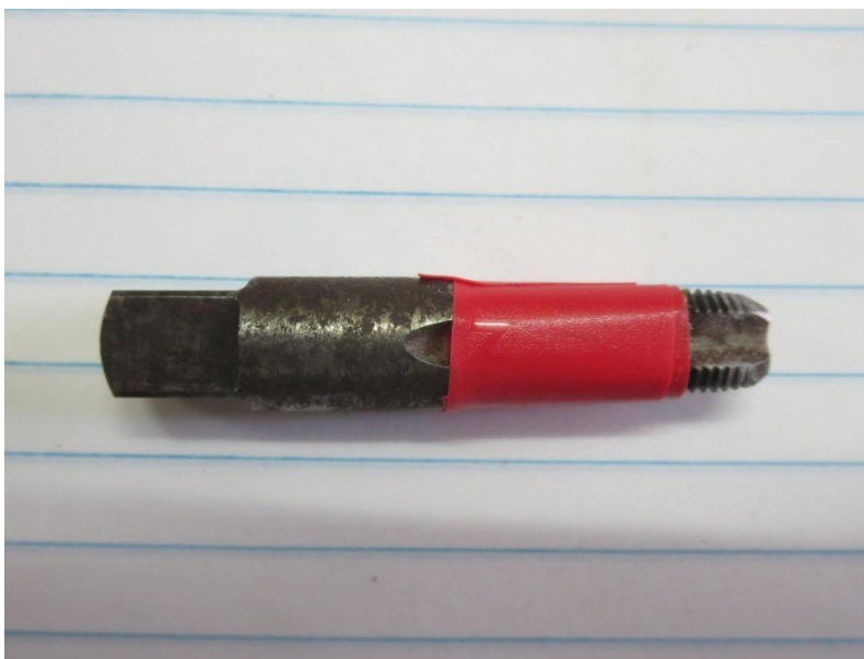
9. 1/8" BSPP tap showing approximate tapping depth from end to tape
