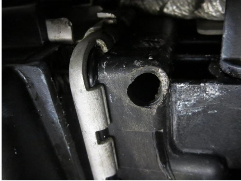
4. Drilled in stages to 11/32" to suit a 1/8" BSPP tap
