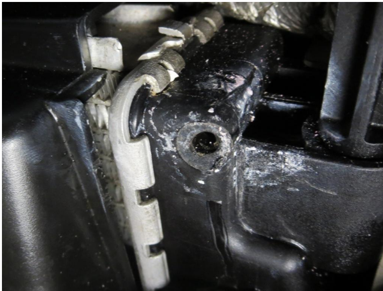
2. The hole left in the radiator was 4mm diameter
