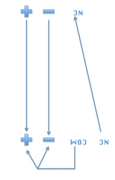
Com to either + or - will depend on which polarity your door closer requires to open on alarm.
