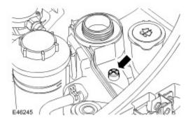
20. Loosen the cylinder head bleed hose bleed screw.
