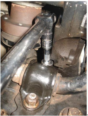
You will only be able to use the socket for a couple of turns before it gets trapped onto the nut by the diff bracket. Before this happens you will need to take the socket off and use an 18mm open ended spanner.....
