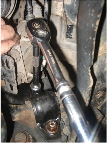
To get the ARB bracket nuts released initally I used a 1/2" breaker bar with 1/2 to 3/8 adapter, short 3/8 extension and 3/8 18mm socket. That gave enough leverage, which a 3/8 ratchet drive didn't.
