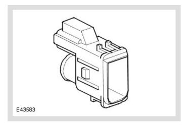
The in-vehicle temperature sensor is a NTC thermistor installed behind a grill on the driver side of the center console finisher. The sensor is connected to a tube, the other end of which is connected to a venturi on the side casing of the heater. An air bleed from the heater, through the venturi, induces a flow of air down the tube, which draws cabin air through the grill and over the sensor.
