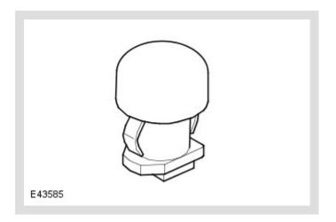
The sunlight sensor consists of two photoelectric cells that provide the ATC module with inputs of light intensity, one as sensed coming from the left of the vehicle and one as sensed coming from the right. The inputs are a measure of the solar heating effect on vehicle occupants, and are used by the ATC module to adjust blower speed, temperature and distribution to improve comfort. The sensor is installed in the center of the fascia upper surface and is powered by a 5V feed from the ATC module.
