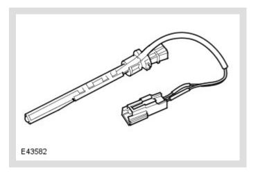
The evaporator temperature sensor is a NTC thermistor that provides the ATC module with a temperature signal from the downstream side of the evaporator. The evaporator temperature sensor is installed in the right side of the heater assembly casing.
