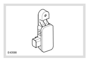
The pollution sensor allows the ATC module to monitor the ambient air for the level of hydrocarbons and oxidized gases such as nitrous oxides, sulphur oxides and carbon monoxide. The sensor is attached to a bracket on the front-end carrier, at the top left corner of the condenser.
