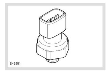
The refrigerant pressure sensor provides the ATC module with a pressure input from the high pressure side of the refrigerant system. The refrigerant pressure sensor is located in the refrigerant line between the condenser and the thermostatic expansion valve.
